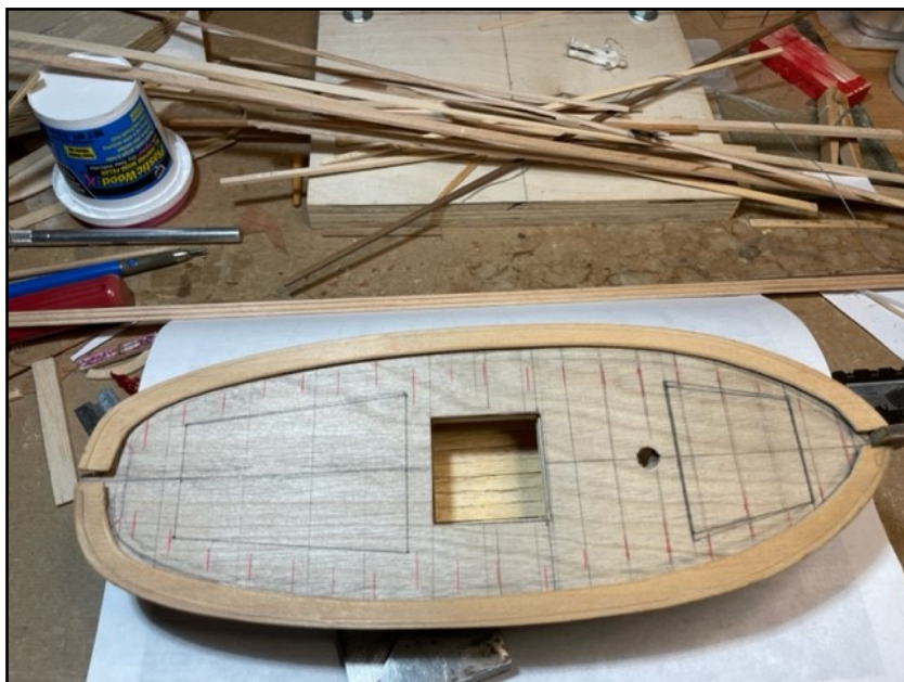
False deck and cover boards ready to be installed.
